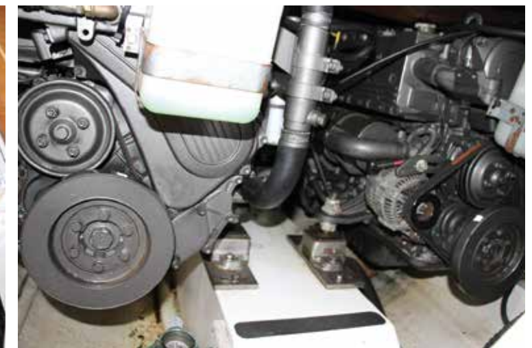
Left, Yamaha ME 420 DTi's fitted to a '95 boat. Right, 315hp Yanmar 6LPA/STD's fitted to an '04 320
