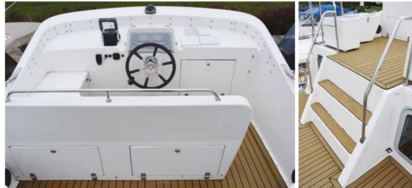
Moulded, narrow-tread steps lead up to the flybridge. Seating configurations vary, 90's boat pictured
