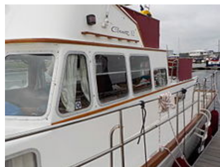
Corvette 32 probably from 1985 showing early half-height side window In later models this was full height
